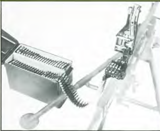
Belt Feed Group has predominantly rolling parts which eliminate sliding friction and gives more than sufficient power to pull 125 rounds of belted ammunition vertically.
