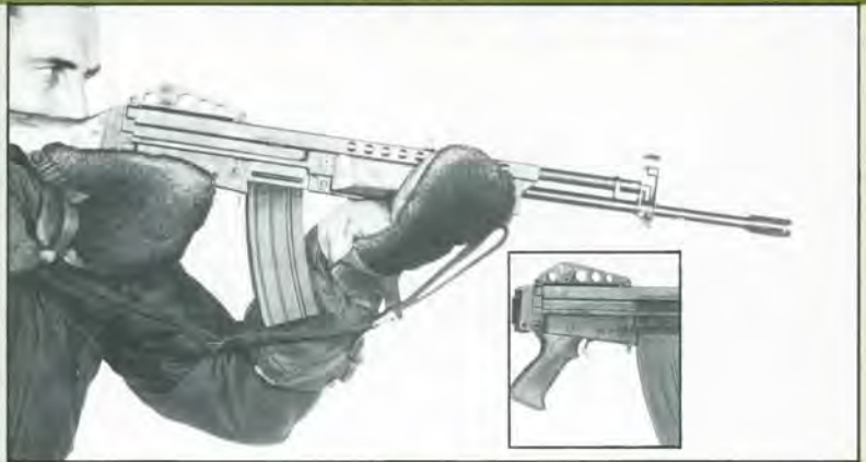
The "winter trigger" feature of the STONER 63 Weapons System permits firing even while wearing arctic gloves by simply removing the spring-steel trigger guard.
