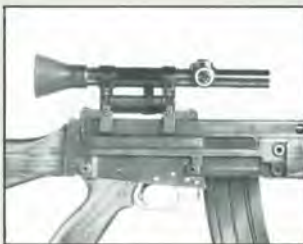
Scope sight readily replaces rear Rifle sight by means of a quick-change mount that provides a stable platform.
