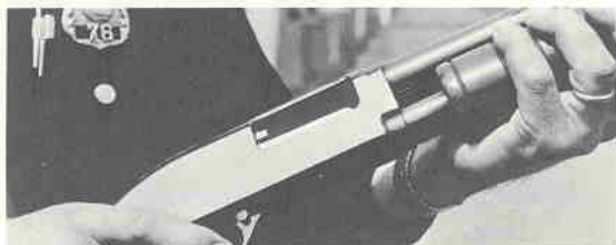
Check the open breech for yourself, keeping finger off trigger.
