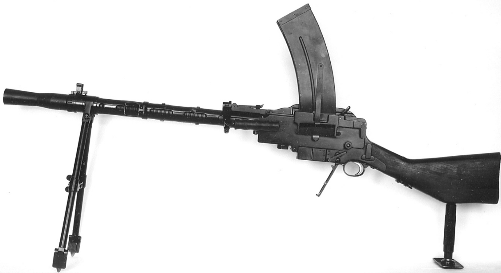
41930 10-28-40 ABERDEEN PROVING GROUND Ordnance Dep't. Madsen 7 mm light machine gun on bipod and stock rest.
