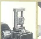
REAR SIGHT-MACHINE GUN folding-leaf type sight, adjustable in \frac{1}{8} -mil increments for windage and elevation, with range scale graduated in 100-meter increments
