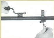
ADJUSTABLE GAS VALVE The adjustable gas valve on the Stoner 63A Automatic Rifle or Machine Gun Barrel gives you three different gas ports to accommodate variations in ammunition
