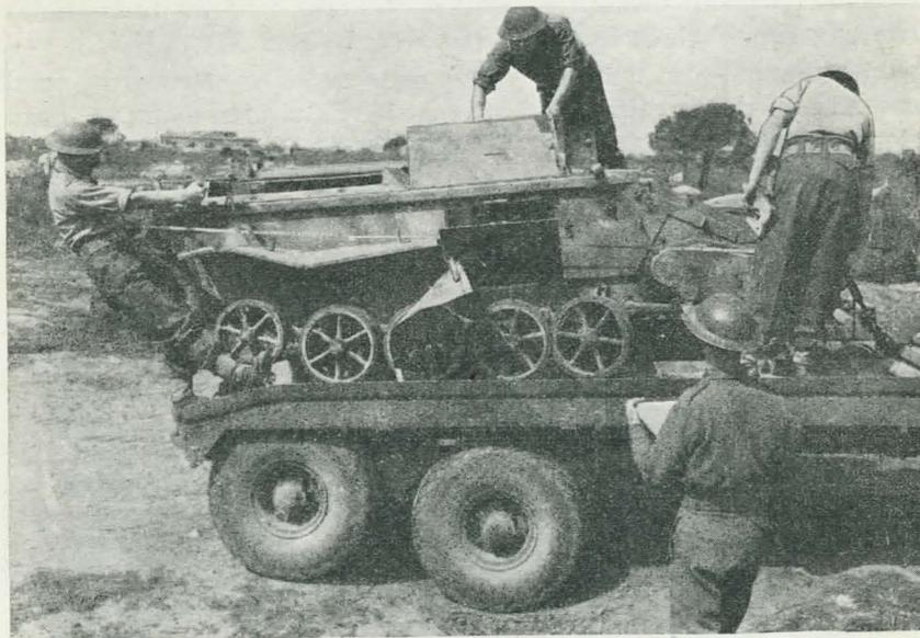
THE B-4 RADIO-CONTROLLED DEMOLITION VEHICLE.
