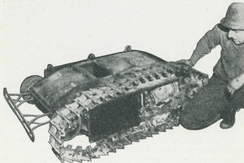
A DAMAGED GOLIATH, LINE-CONTROLLED DEMOLITION VEHICLE.
