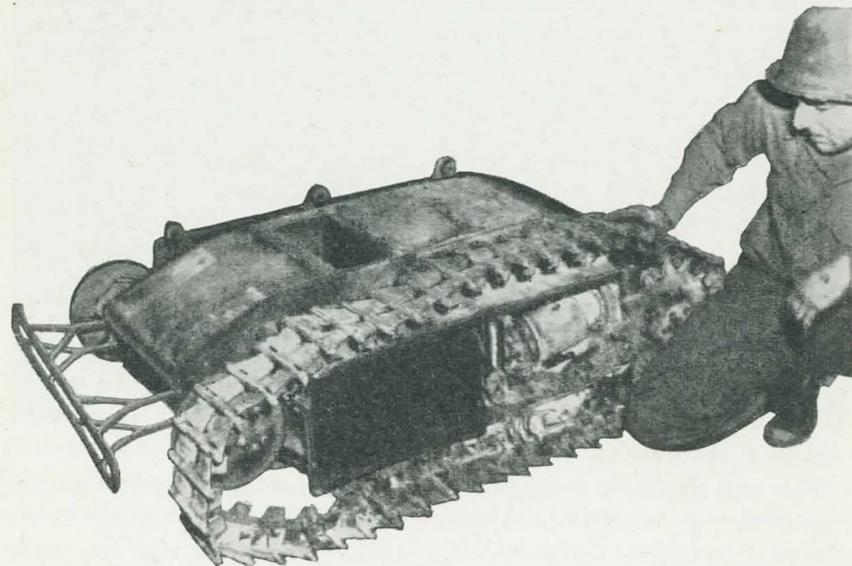
A DAMAGED GOLIATH, LINE-CONTROLLED DEMOLITION VEHICLE.
