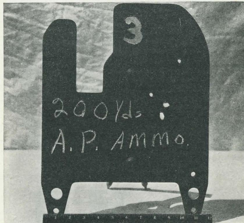
PHOTO SHOWS 4 PENETRATIONS OF ARMORED SHIELD BY ARMOR PIERCING AMMUNITION FIRED FROM RIFLE AT 200 YARDS RANGE.
