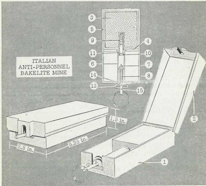
To neutralize the mine, carefully lift the lid clear of the actuating pin (13). Place a wire in inner hole (15) and lift out the whole striker assembly. Unscrew the locking ring (11) and take out the detonator.
