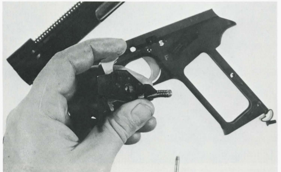
This little unit contains most of the fire control apparatus, includes window to lubricate through. A screw holds this in place in Gunfacts' sample gun.
