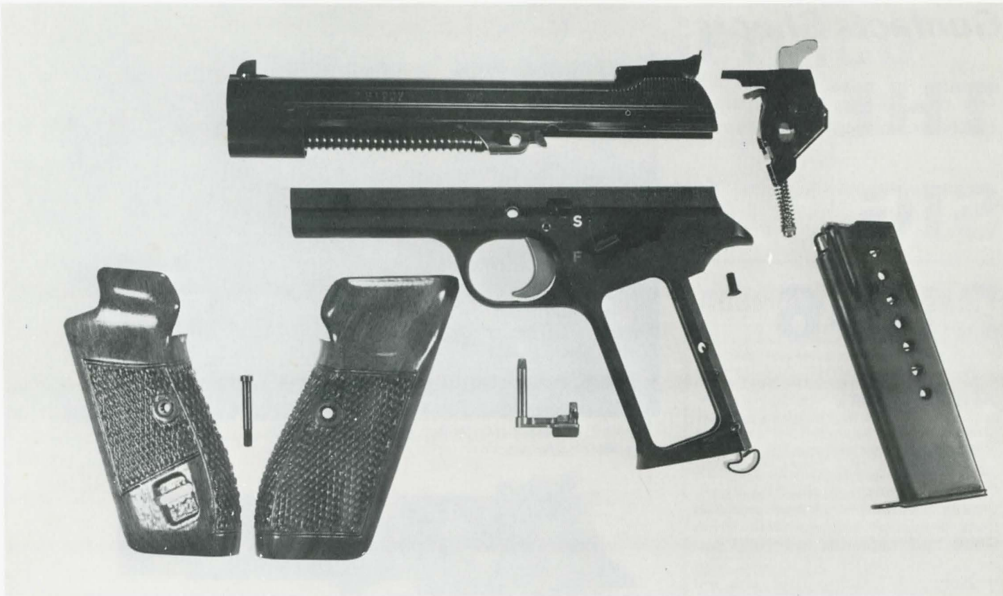
The stripped SIG 210-6 looks like this. Barrel is left in slide to show basic Browning approach. Unitized hammer group is non-Browning, of course. Note long track on slide, which houses inside frame.
