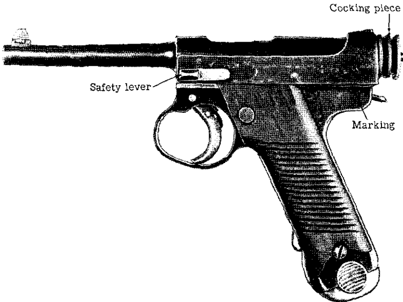
Figure 8.—Model 14 (1925) 8-mm pistol (left side).
