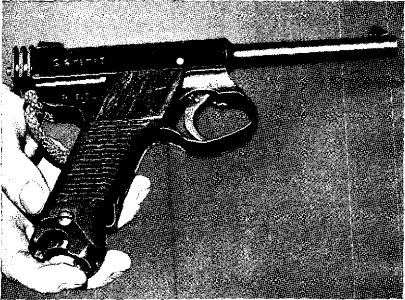
Figure 11.—Model 14 (1925) 8-mm pistol (right side), showing lanyard.
