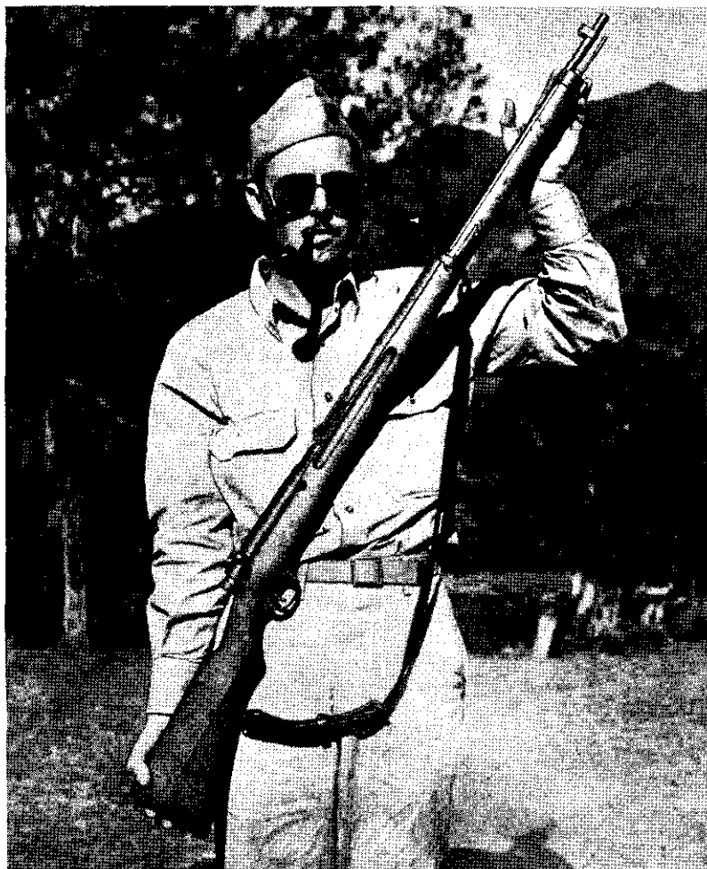
Figure 17.—Model 38 (1905) 6.5-mm rifle, showing its unusual length.
