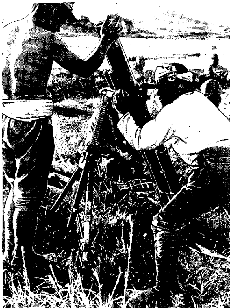
Figure 99.—Laying-in Model 94 (1934) 90-mm mortar.
